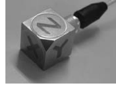
Figure 3 : A photo of an acceleration scales to measure three degrees-of-freedom accelerations along X, Y and Z axes.
